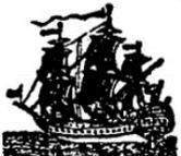
**THE SARAH** Brigantine, a Prime Sailor, Square-stern'd, Plantation-Built, Burthen 120 Tons, more or less, Length by the Keel about 56 Foot, Breadth by the Beam about 20 Foot 6 Inches, Depth in the Hold about 10 Foot, Height between Decks about 3 Foot 10 Inches, now lying upon Mr. Smith's Ways, a little below the Hermitage, John Skinner, late Commander.
